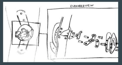
The most important aspect of the hinge systems discussed, independent of which is chosen, is the placement of the hinge system. The hinge must be placed adjacent to the wearer's knee. Misplacement of the hinge can lead to user varying degrees of injury, irritation, etc. [10]
