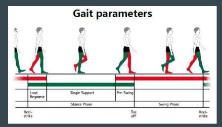
Phases of the gait cycle when walking and the associated loads during each phase
