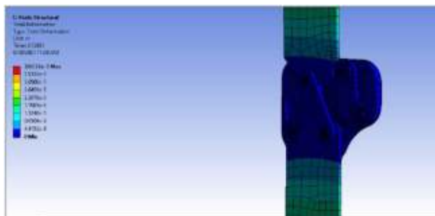
Figure 21. This figure shows the deformation of the hinge design during normal loading. The results showed a maximum of 39.8 \mu m
