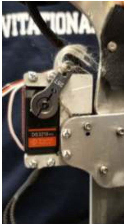
Figure 14. The servo is attached to a threaded string which controls the slider (not seen) for controlled angle restrictions
