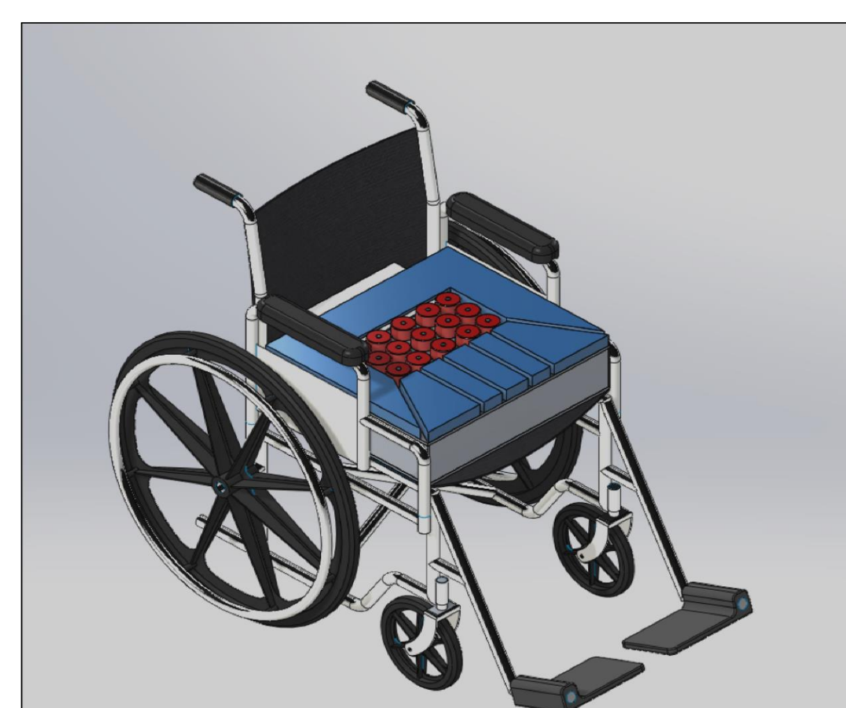
Figure 3. Smart Cushion device mounted on a standard wheelchair. Due to limited budget a prototype displaying proof of concept was constructed. The bladders are only present in the defined area where max interface pressure occurs. A stiff foam encompasses the areas around the maximum pressure to support the rest of the gluteus and legs. The slits in the cushion are to ensure ventilation so the air flow generated thermoregulation
